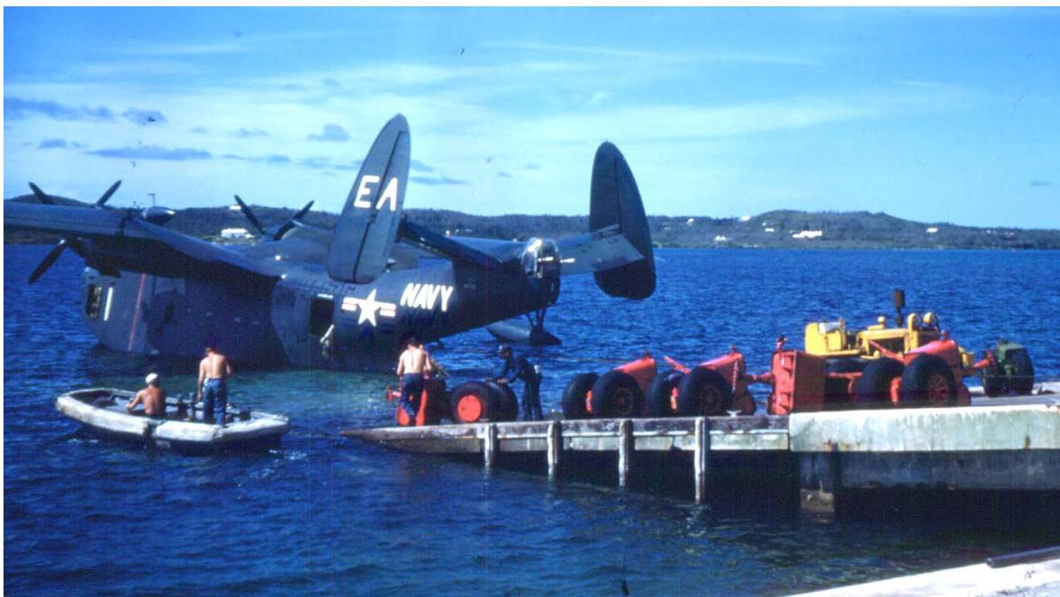
**Seaplanes could land and takeoff only on water. To move them off the water after flight required either a big seaplane tender or a ramp with a buoy for the seaplane to moor while a beaching crew attached removable wheels. Three tractors were required in order to bring a PBM up a ramp. This was a very labor intensive process. Shown here is a seaplane ramp at US Naval Station Bermuda in 1952.**
