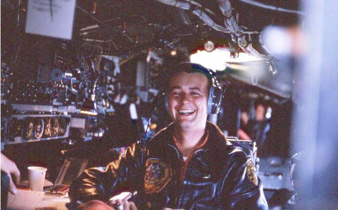
**LTJG Tom Husband at the P2V navigator's station. Note the crowded conditions. The P2V airframe was designed at the end of WWII. The Cold War antisubmarine equipment added later did not fit well in the small P2V interior space.**
