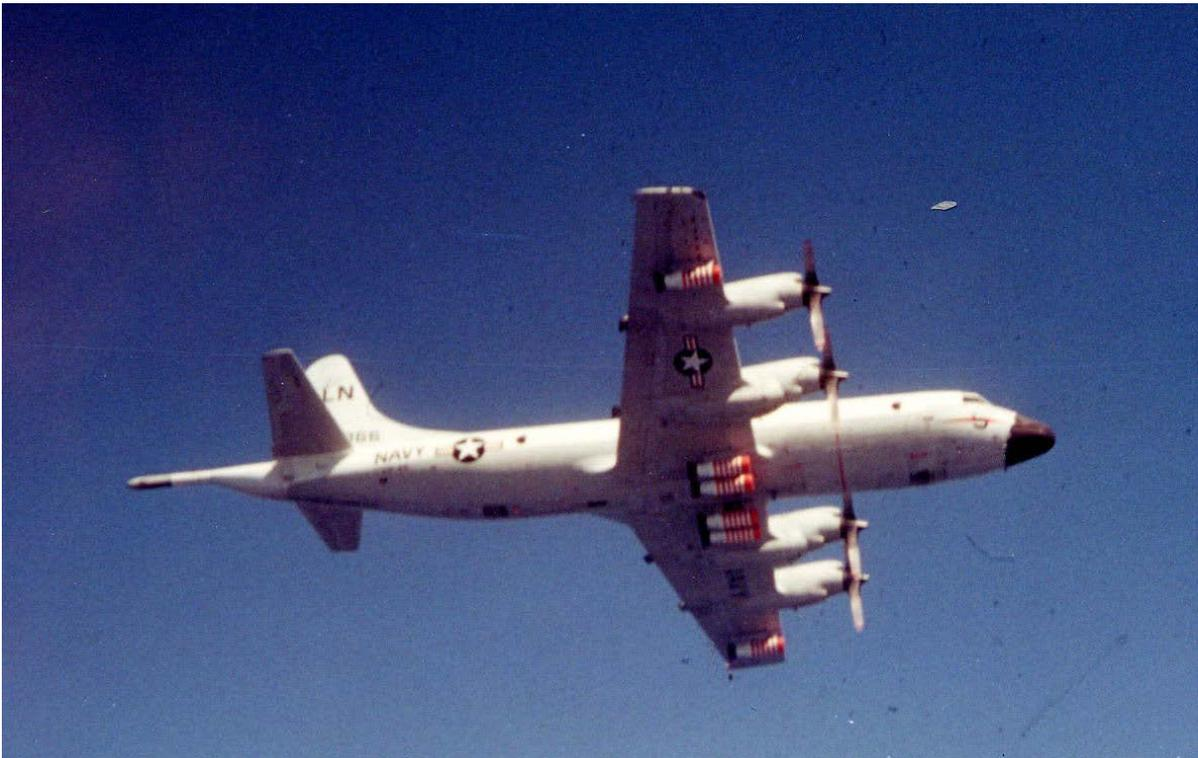
**This photo shows a VP-45 aircraft carrying a 12,000-pound load of mines during an operational readiness inspection in 1967. Accurate placement of the mines under simulated combat conditions was an important test of crew teamwork and precision**
