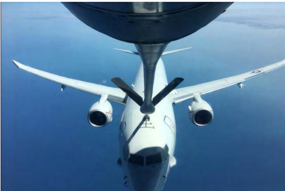
A P-8A Poseidon of Patrol Squadron 45 is refueled while airborne from a KC-135 Stratotanker aircraft from the 909th Air Refueling Squadron April 26 while on a mission in the 7th Fleet Area of Responsibility.
