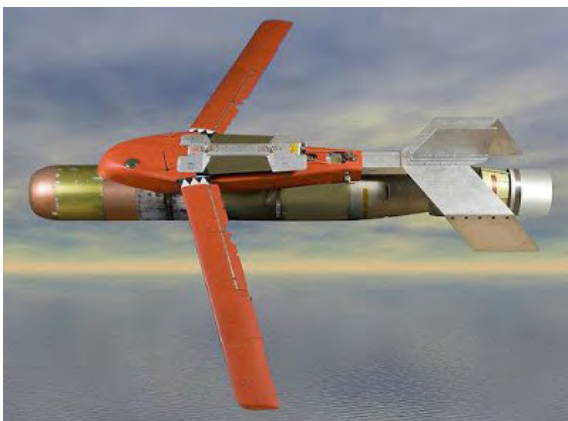
the HAAWC Air Launch Accessory (ALA) for use in launching the Mk 54 torpedo from the P-8A
