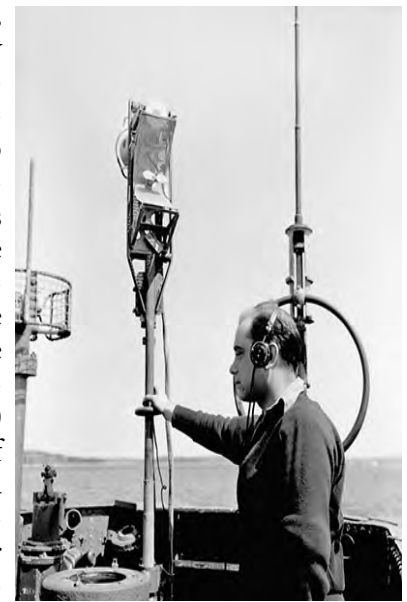
The Naxos radar warning receiver was a World War II German countermeasure to X band microwave radar.
