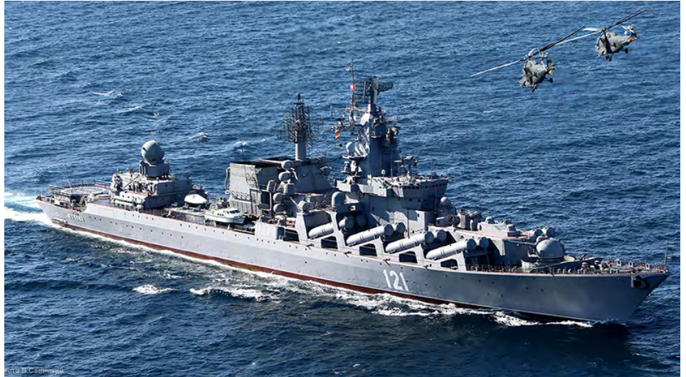
Moskva in her heyday literally bristled with weapons, including 16 anti-ship missiles and 64 long range surface-to-air missiles.
