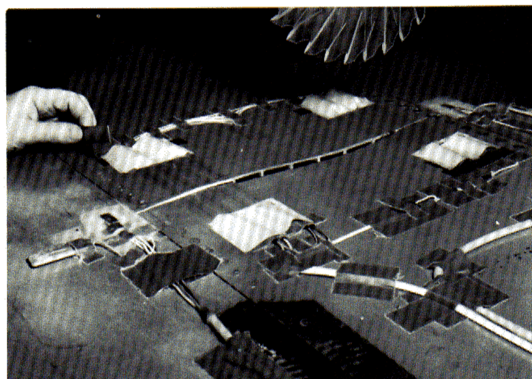
Wing plank saw cut, showing strain gauge installation
