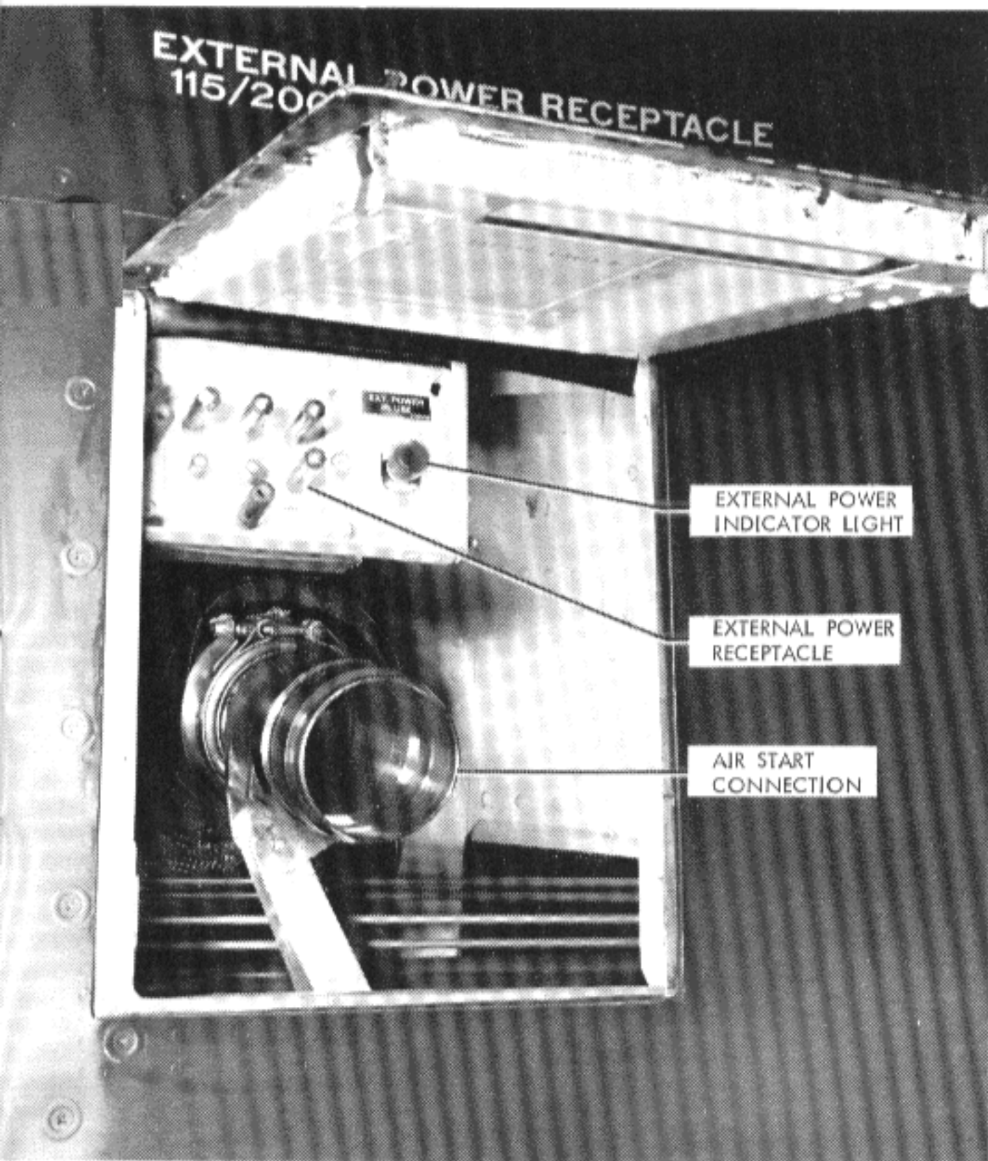
External Ground Power Receptacle
