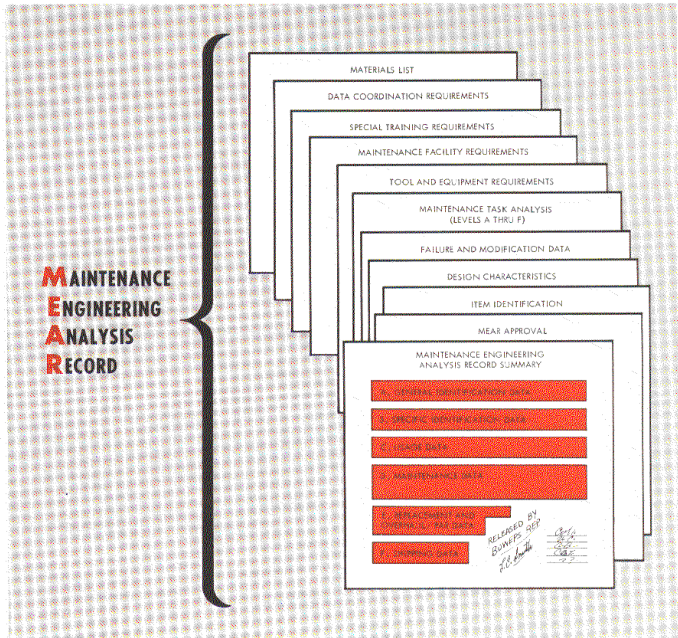
Figure 1 Layout of a Maintenance Engineering Analysis Record
