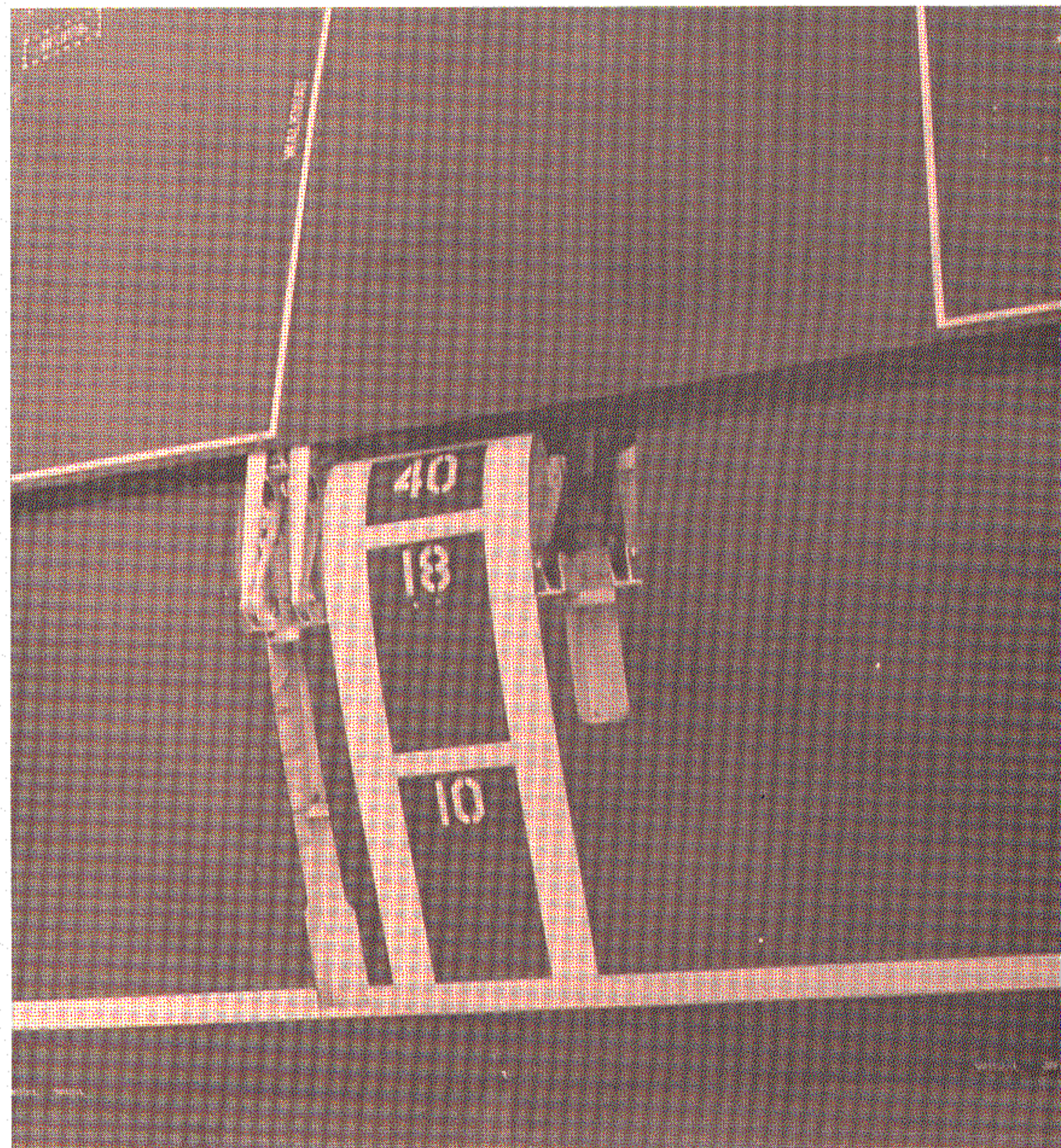
Figure 3 Markings on Wing Flaps Indicate Degree of Flap Deflection — Not Percent of Flap Extension
