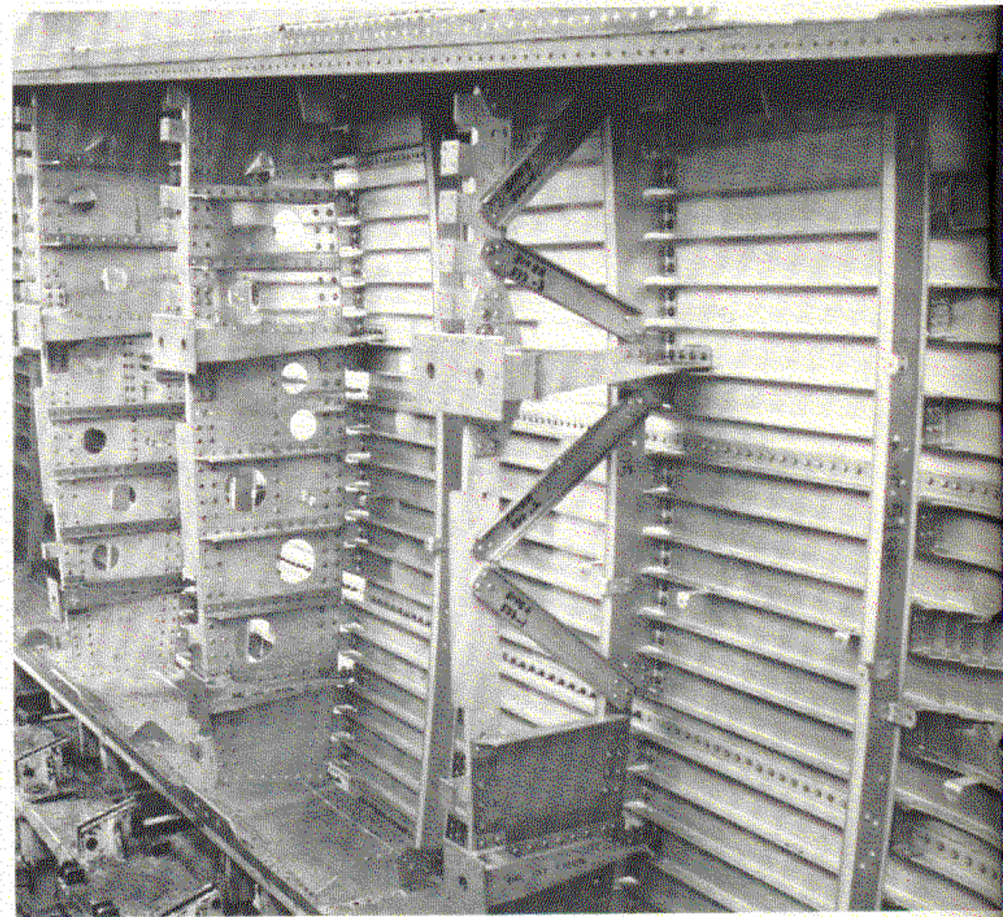
Figure 2 Wing Lower Surface Integrally Stiffened Planks Form the Bottom Surface of the Tanks. Wing ribs and tank bulkheads shown installed.
