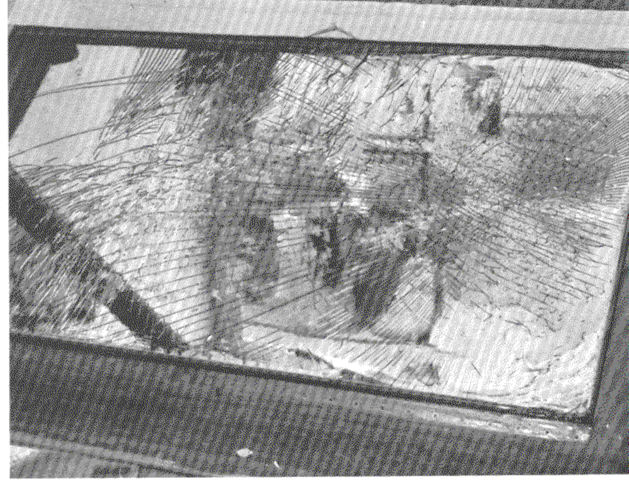
Figure 19. Cold Windshield Tests. Front view of production-type Electra 5-ply windshield panel after impact of a 4-pound bird at 256 knots (vinyl temperature 22°F). Note how cracks radiate from point of impact at top right-hand corner.
