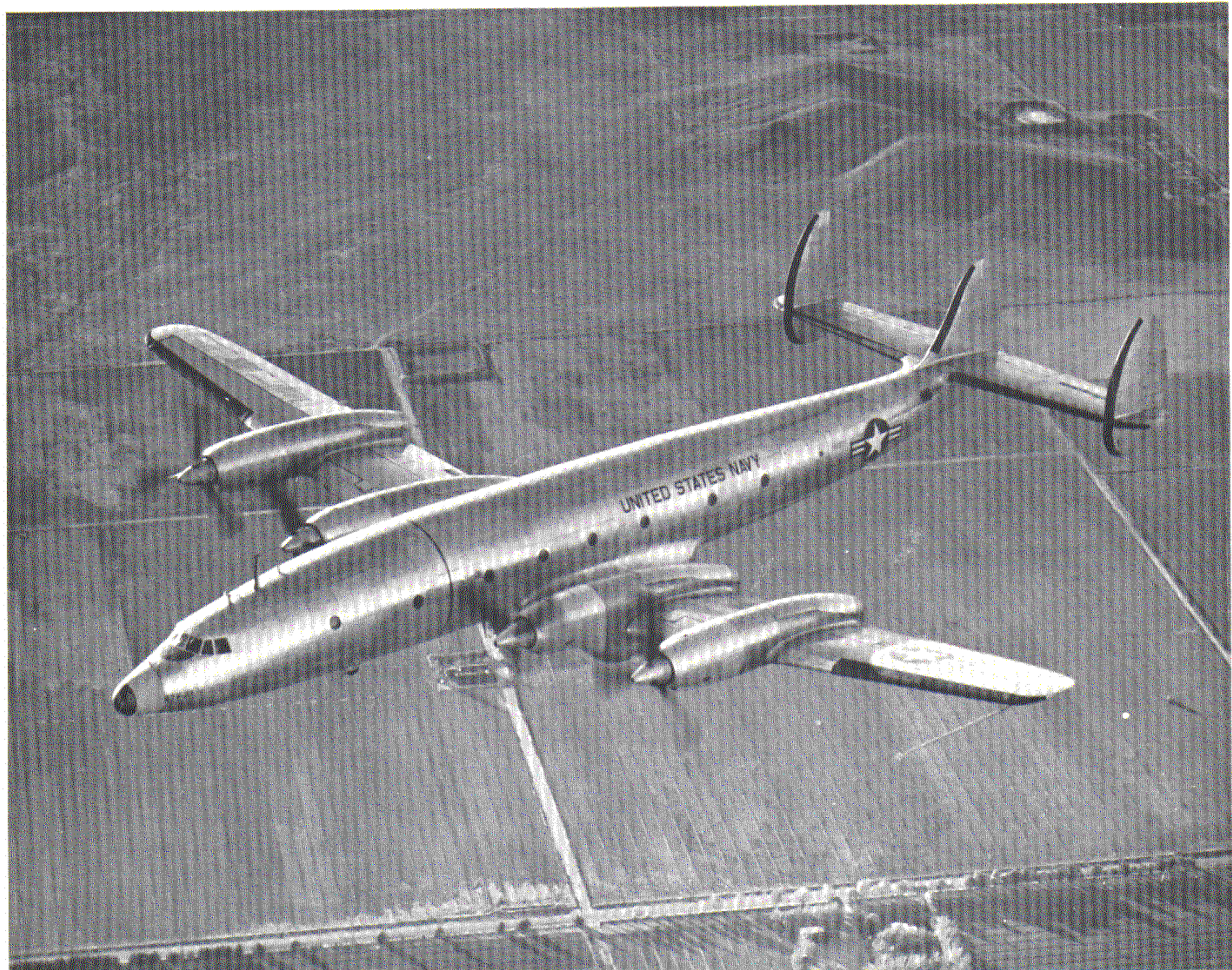
Figure 11. Lockheed R7V-2 Constellation Equipped with T34 Turboprop Engines
