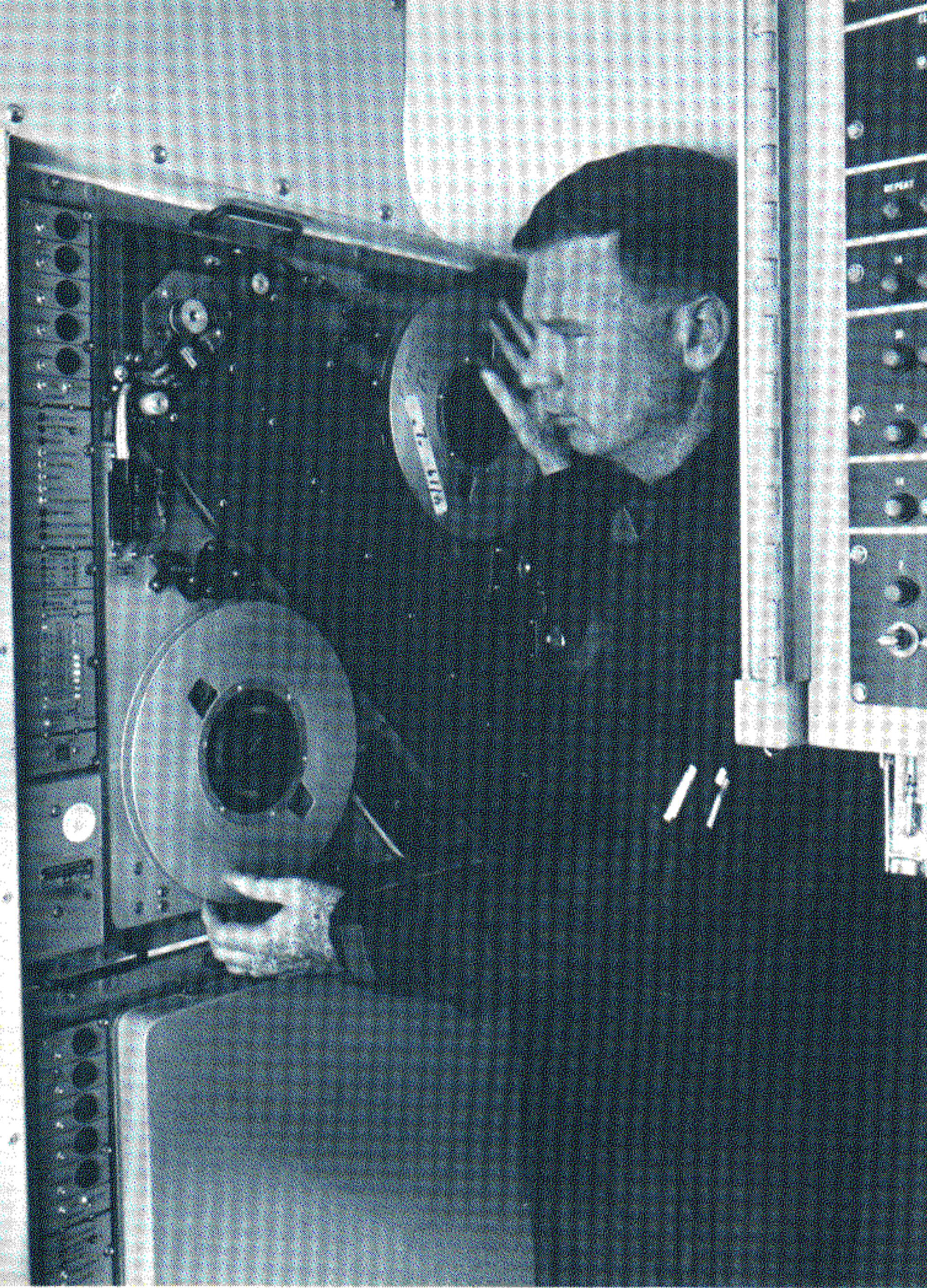
Figure 15. RD-319/AYA-8 Magnetic Tape Transport
