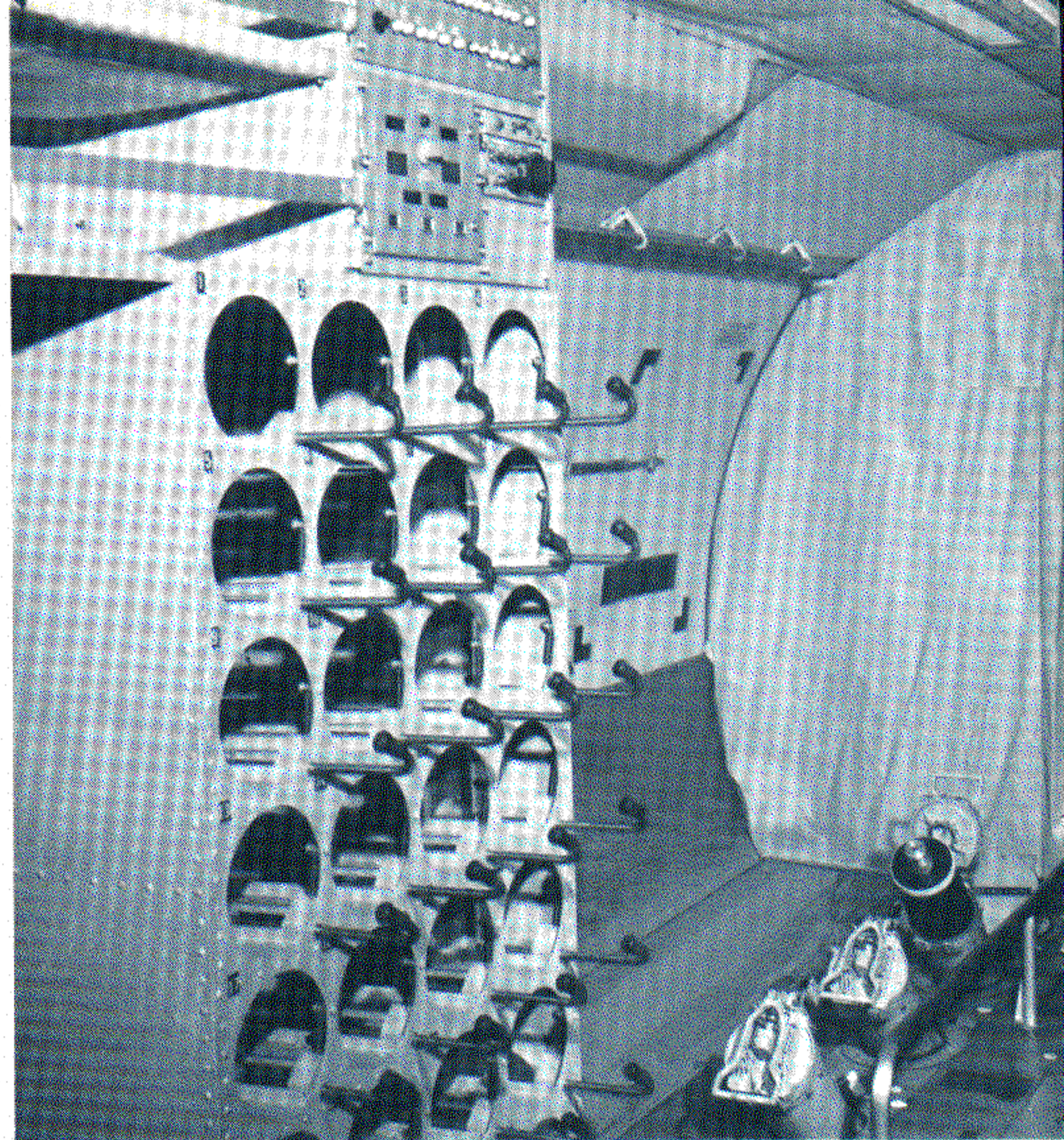
Figure 10. Armament/Ordnance Station. This photograph does not show incorporation of P-3 Airframe Change No. 253 which rotates the hinged breech of the pressurized sonobuoy launch tubes 180°. The new configuration is shown in Figure 30.
