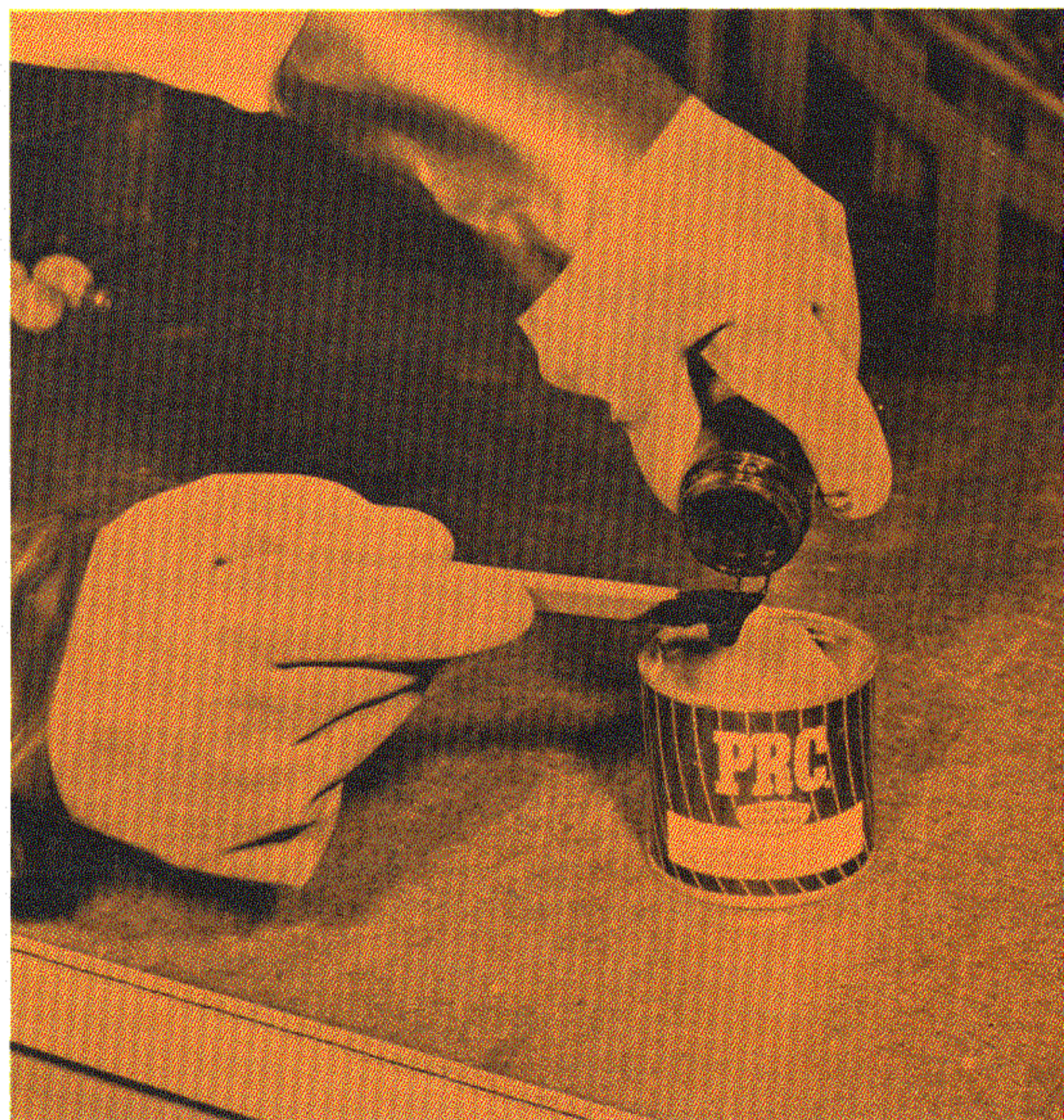
Figure 7. Scrape All the Catalyst into the Base Compound Can and Stir Mixture Slowly by Hand
