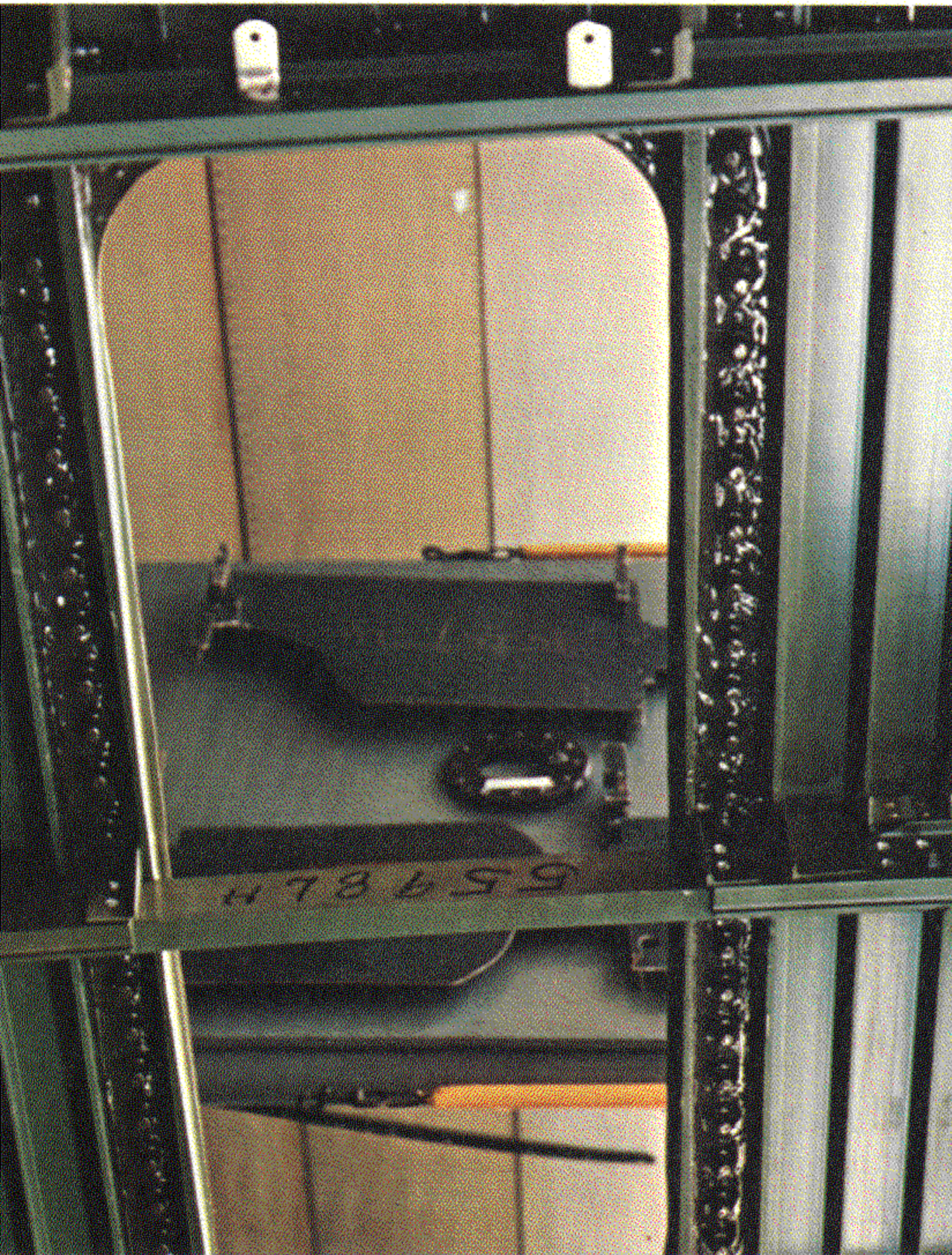
Figure 23. Typical Access Door Opening Showing Sealed Nuts on Door Frame
