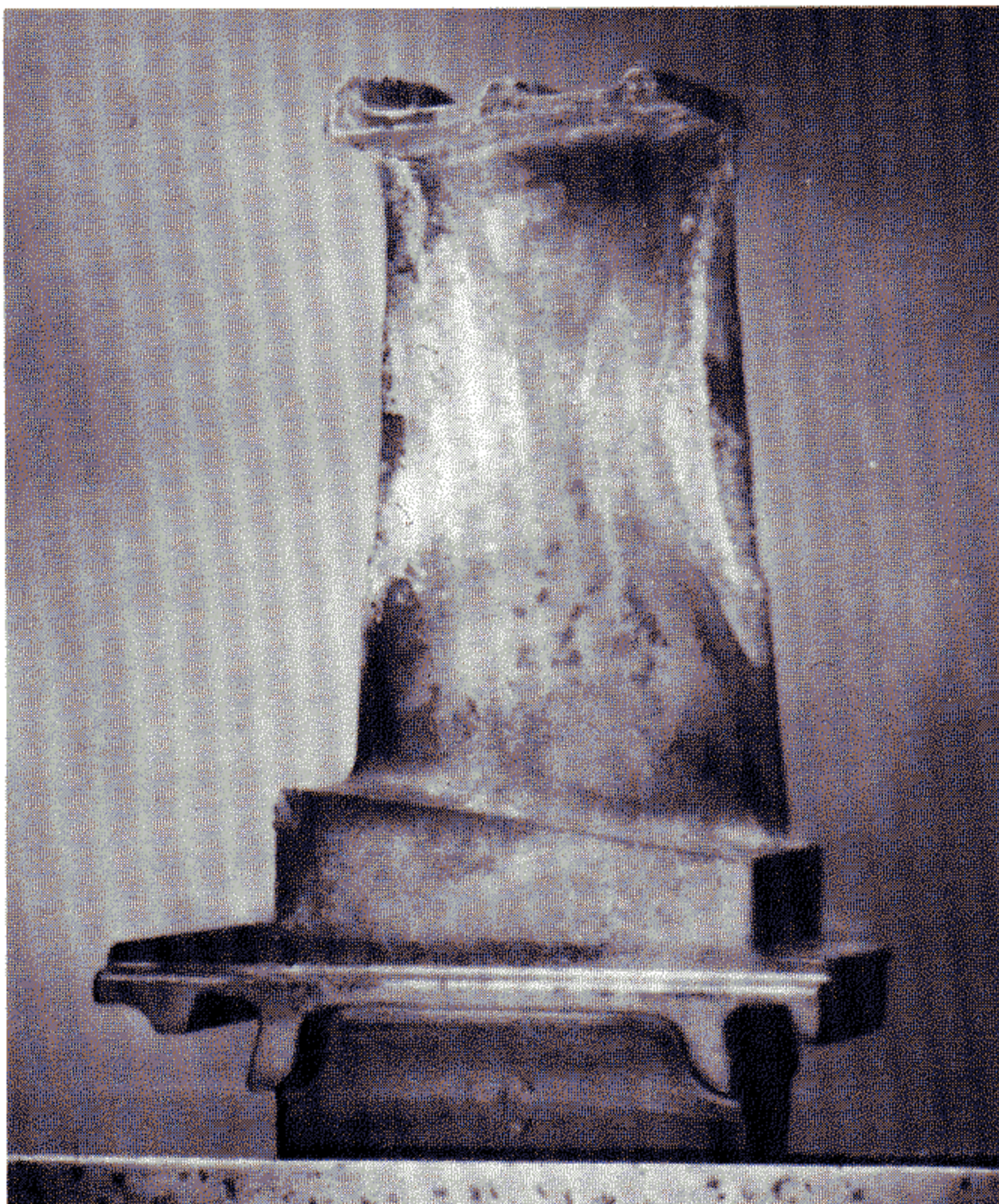
Figure 8 Views of Alpak-Coated Turbine Blade with Sulfidation Damage. Blade was Removed from the First Stage Turbine of a T56-A-14 Engine.
