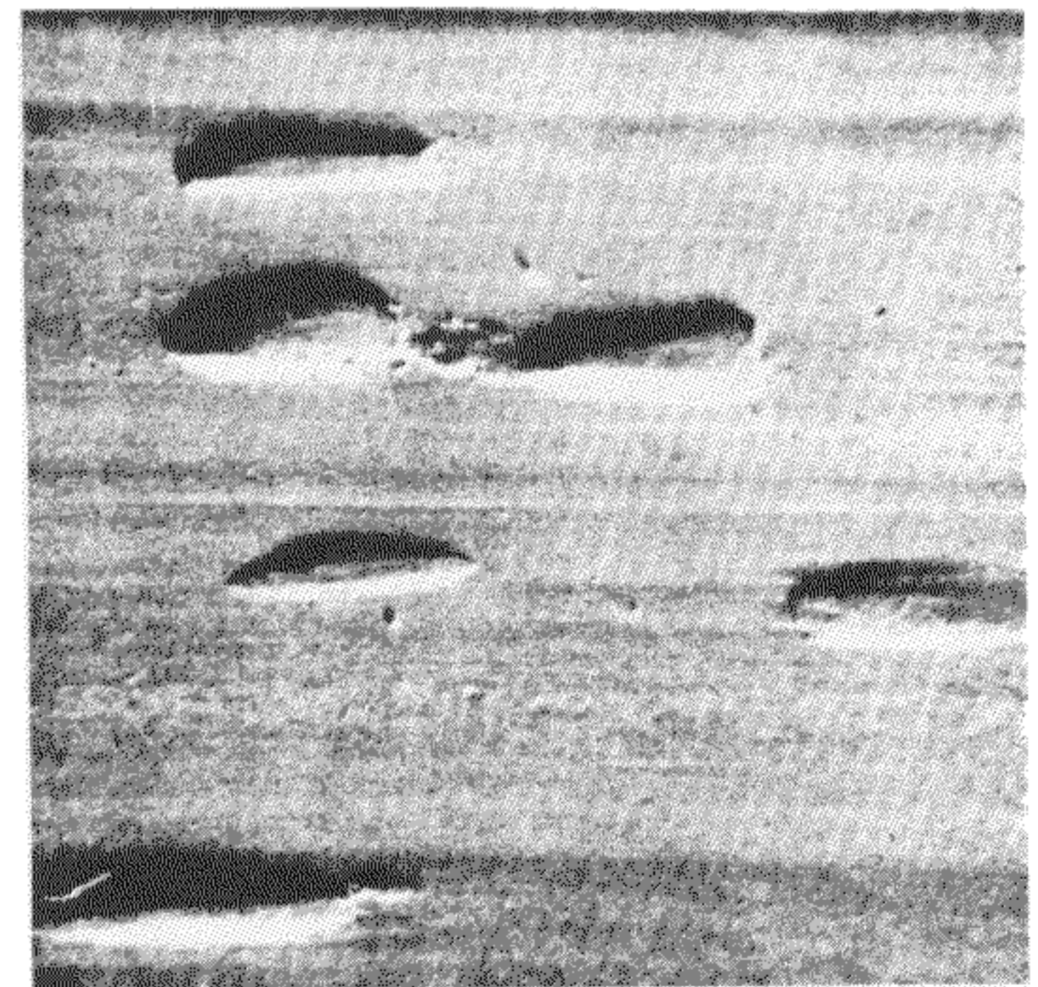
Figure 3. Redeposited Debris on Surface of Well-Worn Tape. Magnified 50X.
