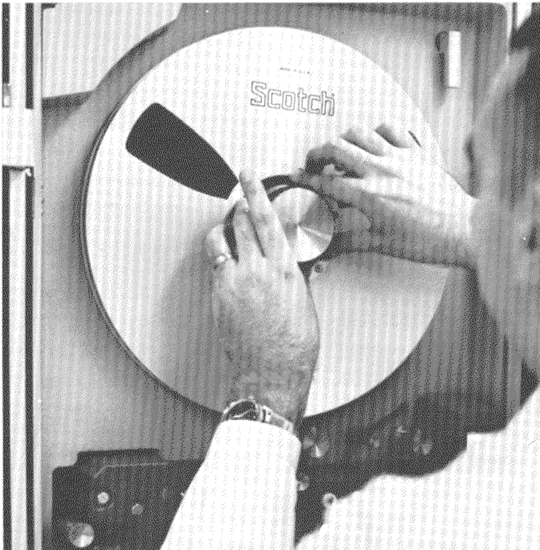
Figure 15. Reel Mounting Procedure.
