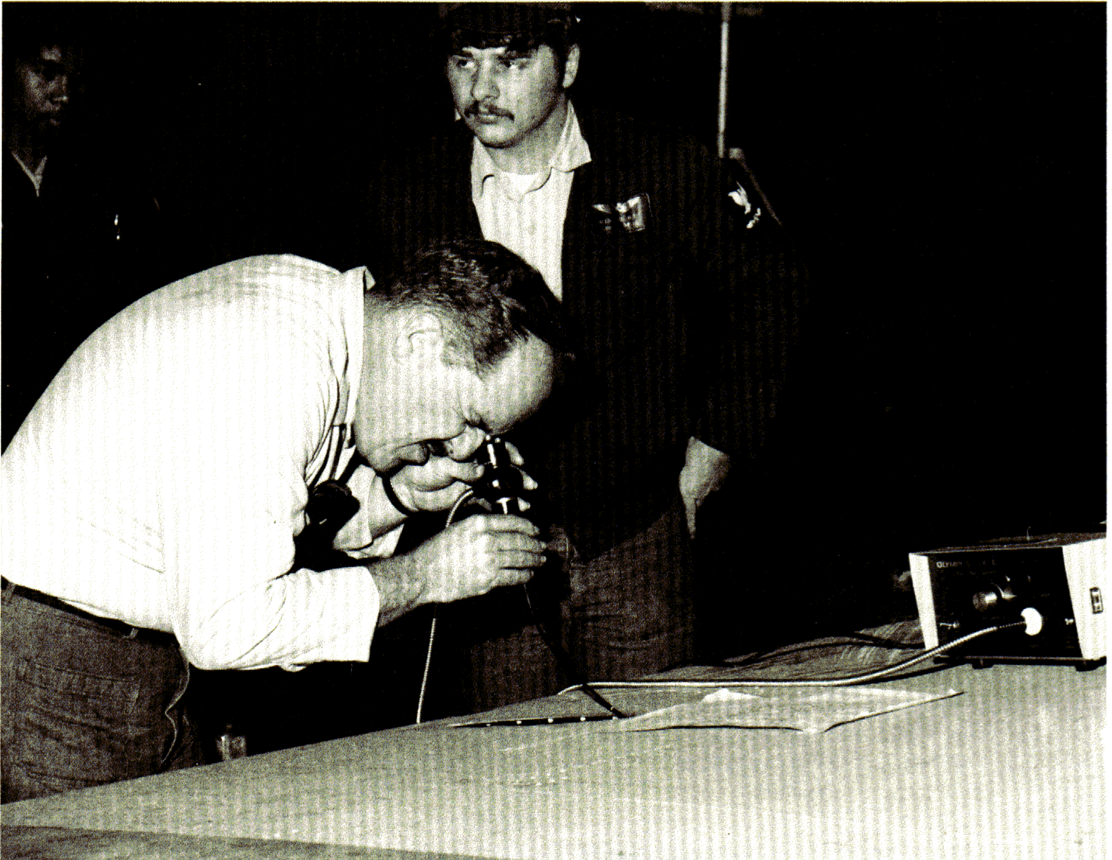
Figure 9. Maintenance Personnel Using 4 mm Fiberoptic Borescope to Inspect Internal Structure of P-3 Wing.
