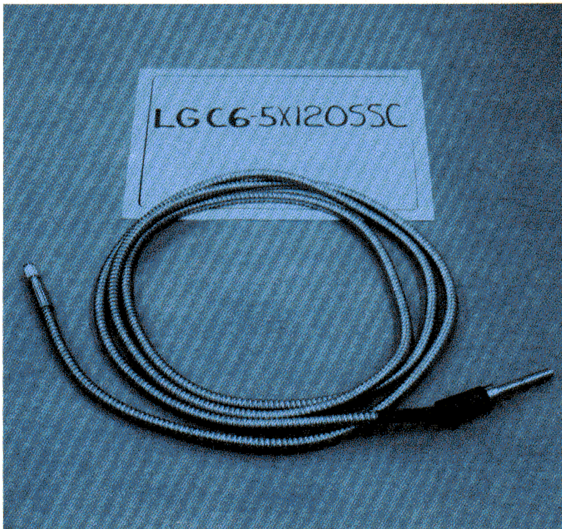
Figure 15. Borescope Light Guide Cable Extension.
