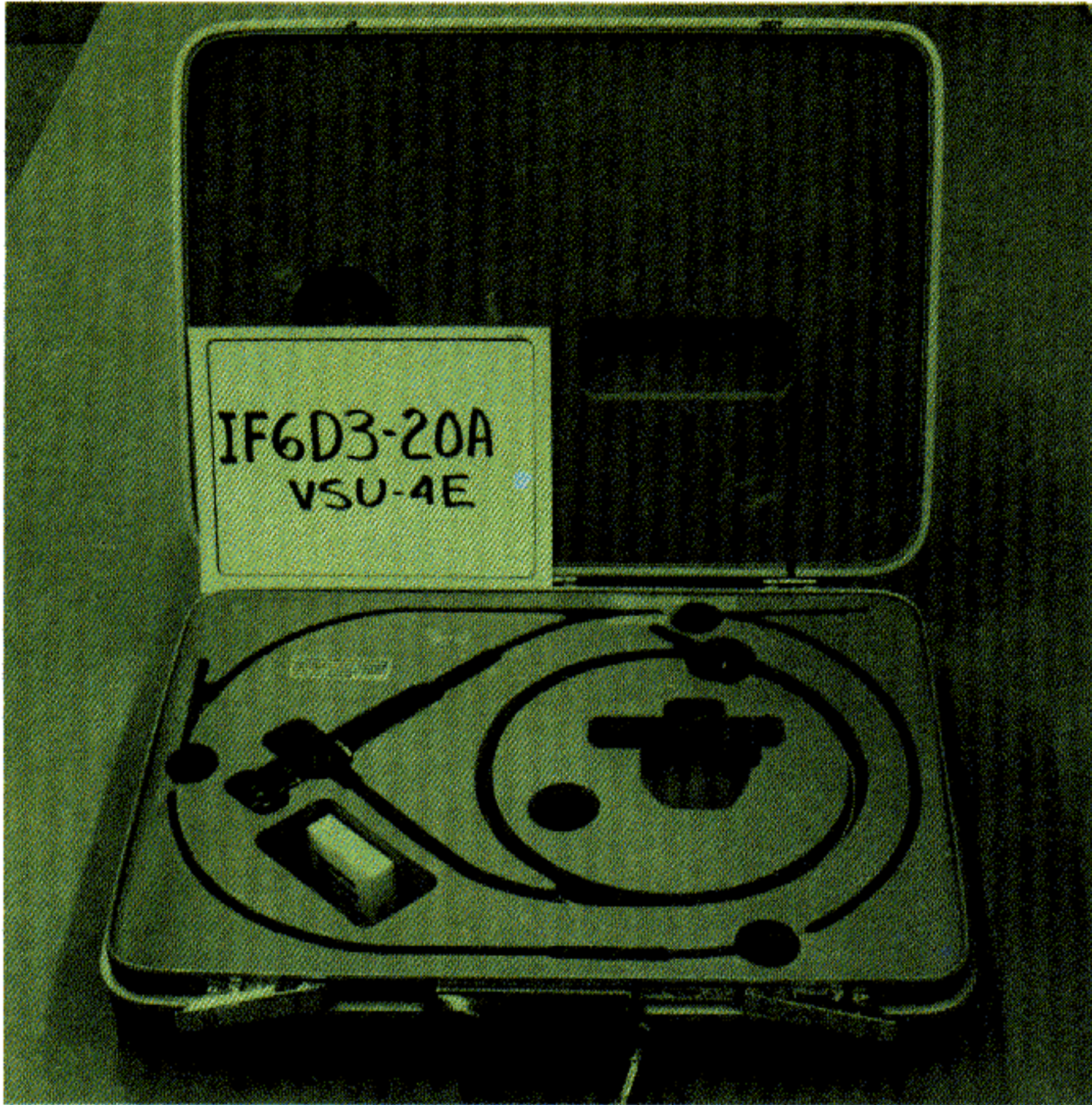
Figure 6. 6 mm Fiberoptic Borescope Stored in Suitcase. Storage of 4 mm and 11 mm Fiberoptic Borescopes is Similar.
