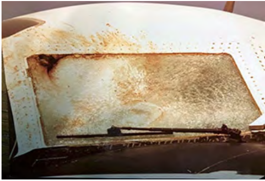
What a good sized bird will do to a perfectly good P-3 windscreen.
